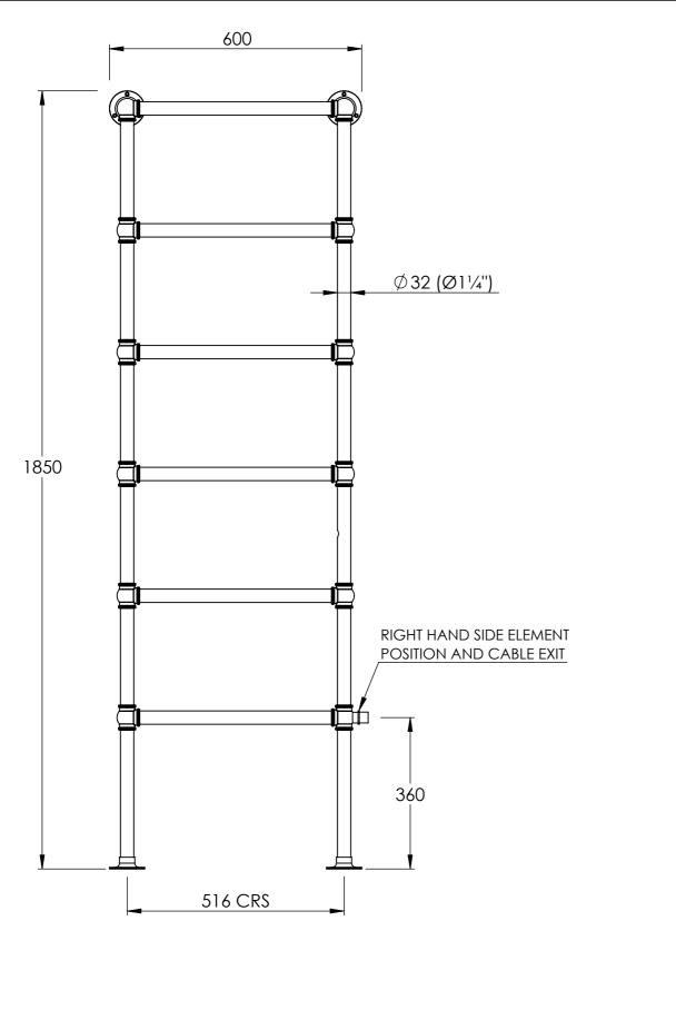
DO NOT SCALE DRAWING ALL DIMENSIONS ARE IN MILLIMETERS AND MAY VARY ± 5mm AS THEY ARE HANDMADE, HAND SOLDERED AND POLISHED
