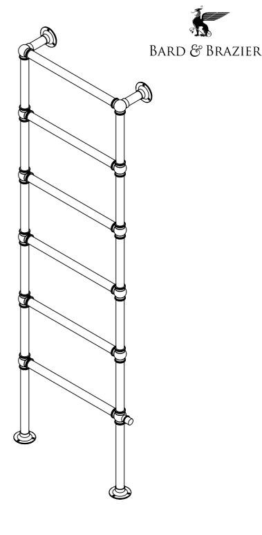
BTU/HR AT DELTA 60: 1819 TEST PRESSURE: ELECTRICAL ELEMENT WATTAGE: 250 MAX WORKING TEMPERATURE:
