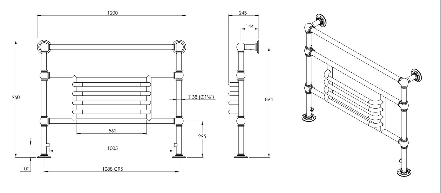
BTU/HR AT DELTA 60: TEST PRESSURE: 4176 CONNECTIONS: FI 1/2" BSP MAX WORKING PRESSURE MAX WORKING TEMPERATURE: HEAT OUTPUT DETERMINED IN ACCORDANCE WITH EN 442 BARD & BRAZIER LIMITED T: +44 (0) 121 270 2222 TITLE: MARSTON ROAD E: INFO@BARDBRAZIER.CO.UK BARONIAL GRILLE FLOOR MOUNTED TOWEL RAIL 950mm x 1200mm - HYDRONIC WOLVERHAMPTON WWW.BARDBRAZIER.CO.UK WEST MIDLANDS
